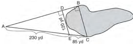
Use the surveyor's information to determine and state the distance from point  $B$  to point  $C$ , to the nearest yard.
