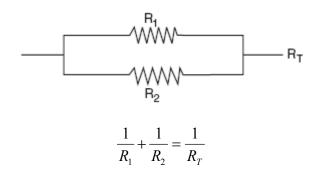
If  $R_1 = x$ ,  $R_2 = x + 3$ , and the total resistance,  $R_T$ , is 2.25 ohms, find the positive value of  $R_1$  to the *nearest tenth of an ohm*.
