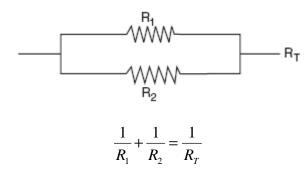
If  $R_1 = x$ ,  $R_2 = x + 3$ , and the total resistance,  $R_T$ , is 2.25 ohms, find the positive value of  $R_1$  to the *nearest tenth of an ohm*.
