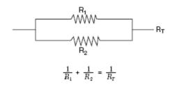
If  $R_1 = x$ ,  $R_2 = x + 3$ , and the total resistance,  $R_T$ , is 2.25 ohms, find the positive value of  $R_1$  to the *nearest tenth of an ohm*.
