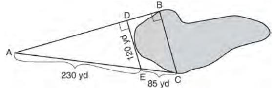
Use the surveyor's information to determine and state the distance from point  $B$  to point  $C$ , to the nearest yard.
