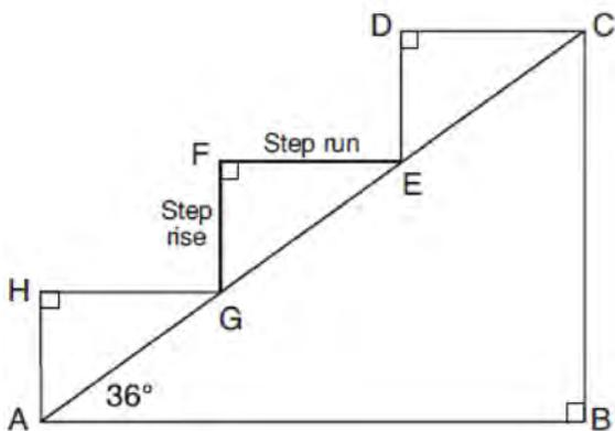
If each step run is parallel to  $\overline{AB}$  and has a length of 10 inches, determine and state the length of each step rise, to the *nearest tenth of an inch*. Determine and state the length of  $\overline{AC}$ , to the *nearest inch*.
